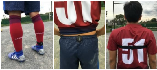
図 2 : Sensor wearing position (inside ankle, lower back, upper back)
